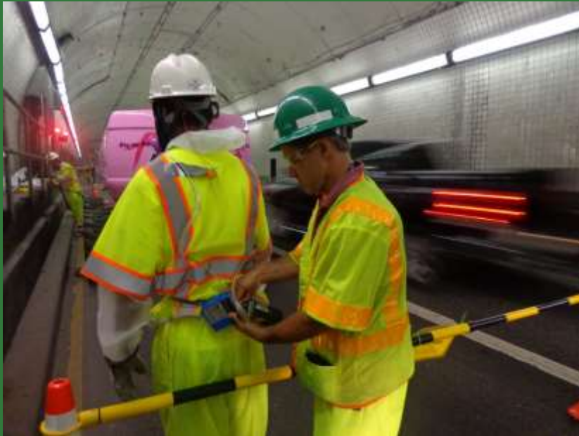
Setting up Sampling Pumps
