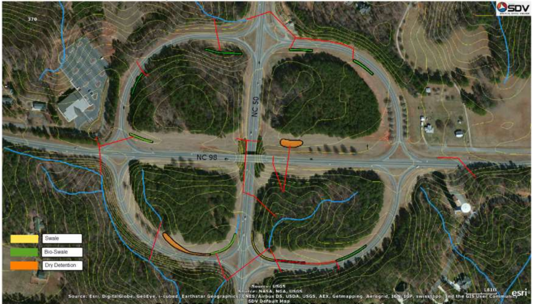
R-4436EG Stormwater BMP Retrofits
